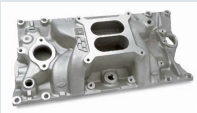
Intake Manifold, Vortec Head Design G
