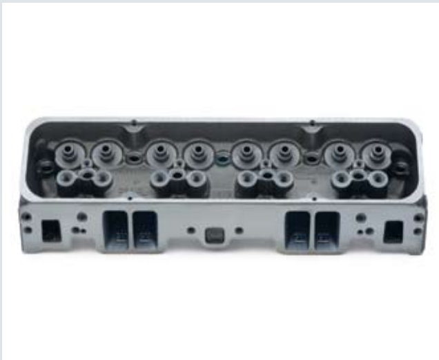
Small and Large Port Vortec Bowtie Heads (intake). B Bare head shown.
