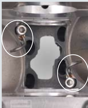
LSA 6.2L Piston Oilers (coolers) B
