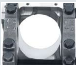
Top—Splayed Main Cap C Bottom—Machined Bottom (close-up)
