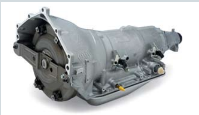
SuperMatic™ 4L85-E Four-Speed Transmission D
