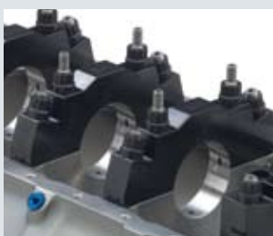
ZL1 Aluminum Big-Block, 4-Bolt Mains B
