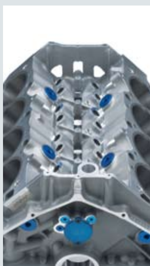
ZL1 Aluminum Big-Block, Lifter Valley B
