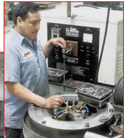
ARP performs the thread rolling operation after heat-treating, which results in a fatigue strength up to 10-times higher than fasteners with threads rolled prior to elevating the material's tensile strength.
