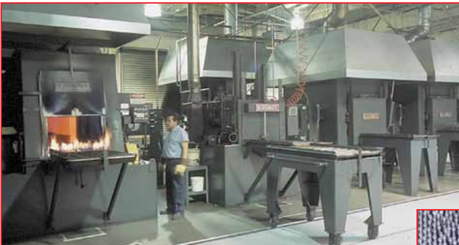
Heat-treating is critically important in obtaining the correct tensile strength. Fasteners are placed in special vertical racks to ensure complete 360° penetration.
