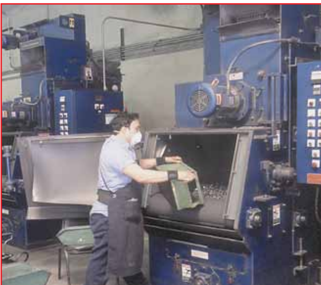
Fasteners are shot-peened after heat-treatment to improve overall external integrity.
