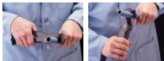
The rotating/rocking technique produces fast easy cuts.
