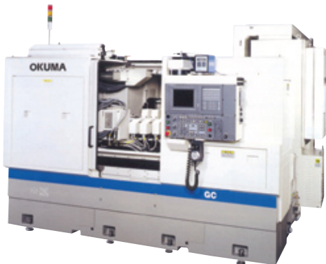
Okuma GC-34 Nh CNC Cam Grinder
