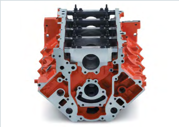
LSX Bowtie Block (front view)
