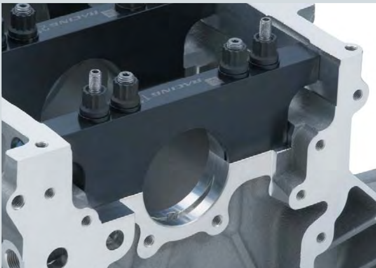
Aluminum C5R Racing Block (main caps) A
