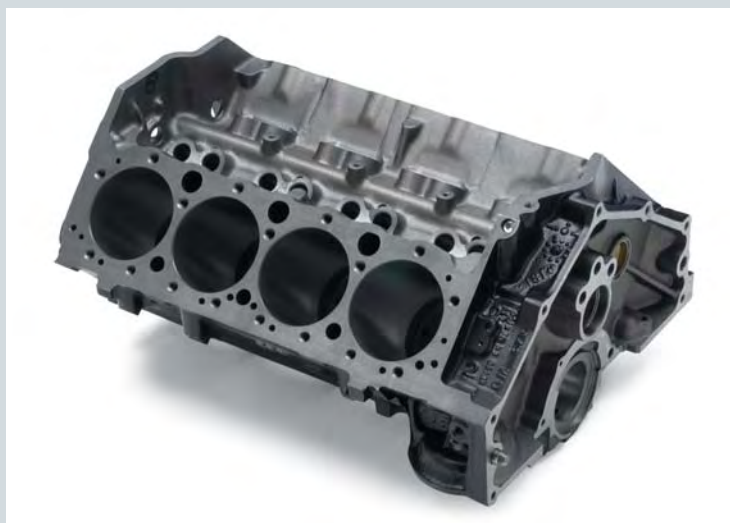
A Two-Bolt Main Block Without Rear Seal Adapter (rear)
